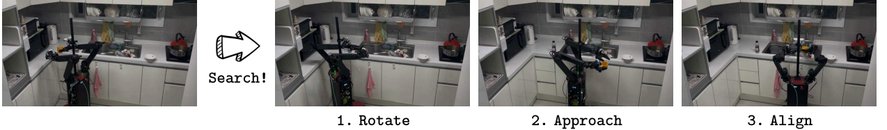
Figure 11. Real-world search behavior. Given only a language prompt and RGB observations, the policy executes searching motions until the sink is visible, then proceeds to complete the task.
